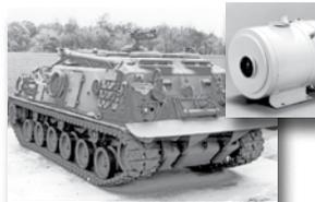
Air Cleaner and muffler on M88A1 Recovery Vehicle
